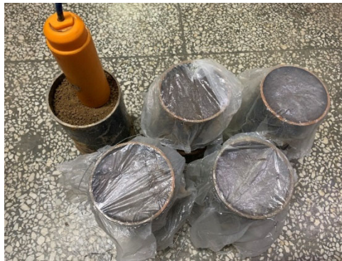
Figure 3. TDR measurement of volumetric water content of single soil sample
