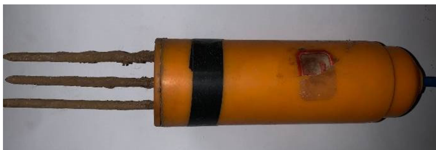
Figure 2: YT-DY-0101 TDR moisture meter
