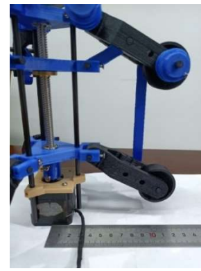
(b) Maximum pipe diameter
